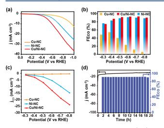
**Figure 3.** Electrocatalytic performance tested in H-cell. (a, b) LSV curves obtained in CO<sub>2</sub>-saturated electrolyte (0.5 M KHCO<sub>3</sub>) and  $FE_{CO}$  over different potentials of the as-fabricated Cu/Ni–NC, Ni–NC and Cu–NC. (c)  $j_{CO}$  of the as-fabricated samples under different potentials. (d) j and  $FE_{CO}$  vs the electrolysis time for Cu/Ni–NC electrode under –0.7 V vs RHE.
