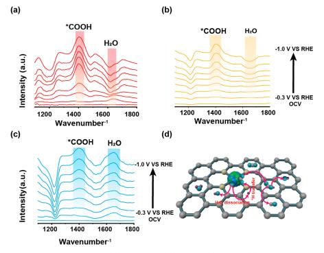
Figure 5. In situ ATR-SEIRAS recorded during  $ECO_2R$  (a) Cu/Ni-NC. (b) Cu-NC. (c) Ni-NC. (d) Proposed catalytic mechanism of Cu/Ni-NC for  $ECO_2R$ .
