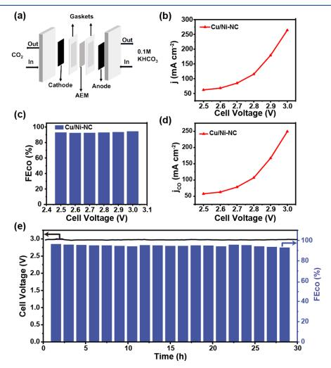
**Figure 4.** Electrocatalytic performance tested in a MEA electrolyzer. (a) Schematic illustration of the electrolysis device. (b) *j* of Cu/Ni–NC under different cell voltages. (c)  $FE_{CO}$  of Cu/Ni–NC under different cell voltages. (d)  $j_{CO}$  of Cu/Ni–NC under different cell voltages. (e) Stability of Cu/Ni–NC electrode under 200 mA cm<sup>-2</sup>.
