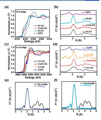
**Figure 2.** Structural characterization. (a, b) XANES spectra of Ni Kedge and FTs of  $k^3$ -weighted Ni K-edge EXAFS data for Cu/Ni–NC, Ni–NC, NiPC and Ni foil. (c, d) XANES spectra of Cu K-edge and FTs of  $k^3$ -weighted Cu K-edge EXAFS for Cu/Ni–NC, Cu–NC, CuPc and Cu foil. (d, e, f) Experimental and the fitting Ni and Cu Kedge EXAFS curves in R space of Cu/Ni–NC.
